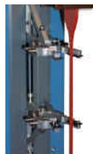
Extensometer arms open to engage with sample
