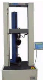
EX800Plus fitted to twin column test machine
