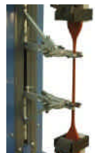
Extensometer arms closed and engaged with sample
